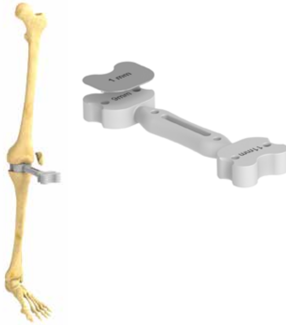
Figure 15 Gap Assessment in Extension with Spacer Block
