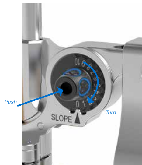
Figure 61 Adjust the Slope Angle by “Push and Turn”
