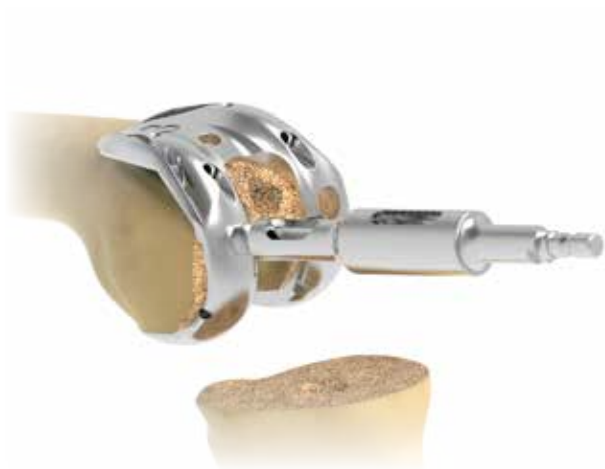
Figure 34 Prepare CR Femoral Peg Hole
